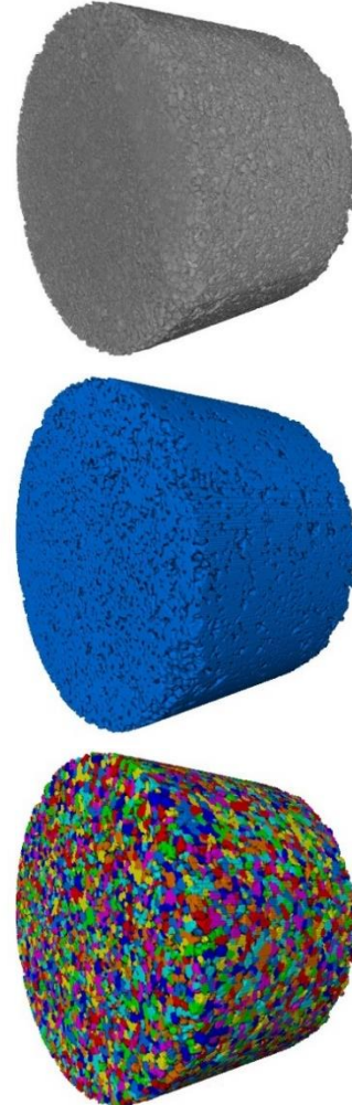
Fig. 1. Construction of sandstone microstructure model in Avizo software: original CT-scan data (top), material segmentation (middle) and particle separation and surface generation (bottom).
