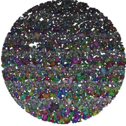
Fig. 2. An example of the 2D numerical microstructure model with a diameter of 10mm.
